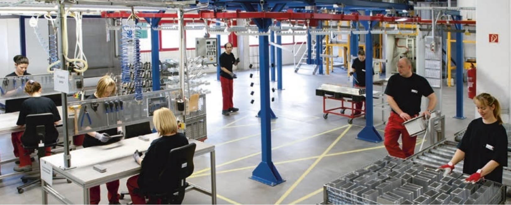
A one-piece flow concept for surface coating has halved the component processing time (above).
